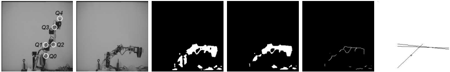
Fig. 2. The ROBIX arm, and the feature points extraction process.
